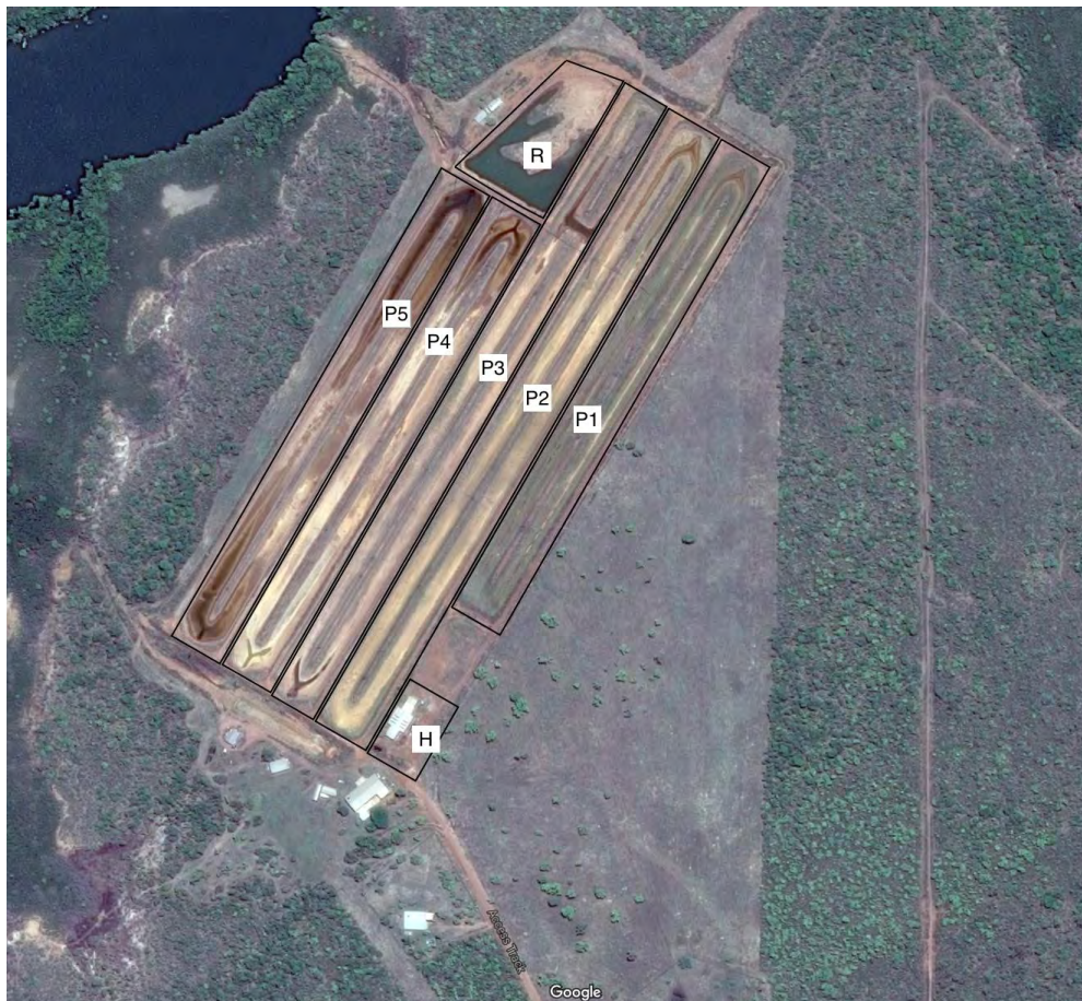
Figure 1. Google Map image of site layout. Site has: 5 raceway ponds (P1= pond 1; P2= pond 2; P3= pond 3; P4= pond 4; P5= pond 5) for grow-out; a hatchery (H) for future breeding and production; and a reservoir pond (R) for recreational fishing.
