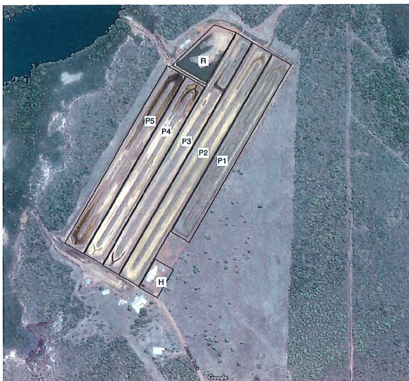
Figure 1. Google Map image of site layout. Site has: 5 raceway ponds (P1= pond 1; P2= pond 2; P3= pond 3; P4= pond 4; P5= pond 5) for grow-out; a hatchery (H) for future breeding and production; and a reservoir pond (R) for recreational fishing.
